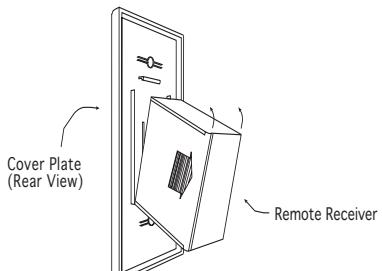
Position the receiver as shown in diagram to the left with lower tab on cover plate inserted into groove of receiver (Make sure LEARN hole on cover plate properly aligns with remote receiver). Pull receiver up and snap into top tab of cover plate.
